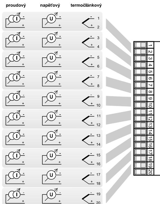
The inputs are *galvanically separated each from other* (and switched over using a relay).
