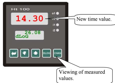
Return from the data logger menu is done by simultaneous depression of the arrow keys.
