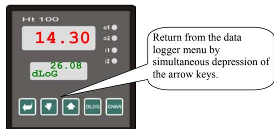
Set the measured value archivation period at the **Operator Level** (parameter
