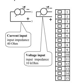
Measuring input is not isolated from the ground of controller
