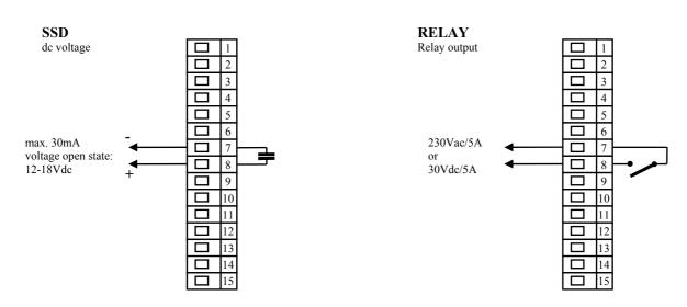
SSD is not isolated from controllers ground
