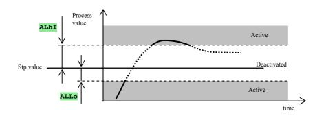
Parameters **ALLO** and **ALHI** define low and high deviation from stp value at which alarm is active.
