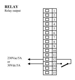
RELAY output is galvanicly isolated from the ground of the controller. For this output it is necessary to fix the wires in the way that in case of loosening the wire from the terminal the insulation would not be reduced between supply voltage and safety voltage.
