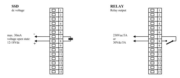
SSD is not isolated from controllers ground
