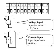
Measuring input *is not galvanic insulated* from the ground of the device
