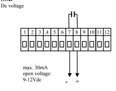
Output SSD *is not* galvanic insulated from the device ground
