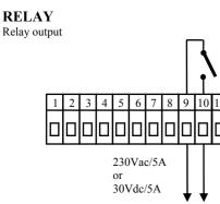
Output RELAY is galvanic insulated from the ground of device. For this output it is necessary to fix the wires in the way that in case of loosening the wire from the terminal, the insulation would not be reduced between supply voltage and safety voltage.
