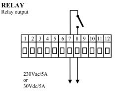
Output RELAY is galvanic insulated from the ground of device. For this output it is necessary to fix the wires in the way that in case of loosening the wire from the terminal, the insulation would not be reduced between supply voltage and safety voltage.
