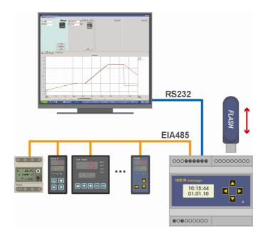
Ht810 can be used as galvanicly insulated convertor RS232 / EIA485.
