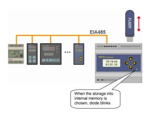
Data are read from the devices that are linked to the line EIA485 and data are stored in the internal memory of datalogger.
