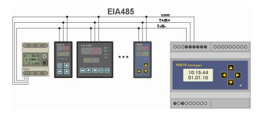
On each device only 1 sole address can be set (range from 1 to 250). Datalogger can be set for reading the measured values from max. 16 devices.
