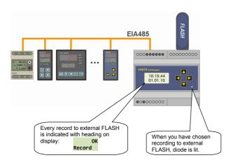
Data are read from the devices connected to line EIA485 and written into internal memory of datalogger and external Flash memory.
