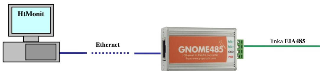
The devices can be linked via this line EIA485 to the convertor. If there are long distances among the devices, one single convertor can be used for each device. In case that it is possible to connect more devices (maximum number is 4) through the communication line EIA485, then you can use one convertor GNOME485 for these devices.
