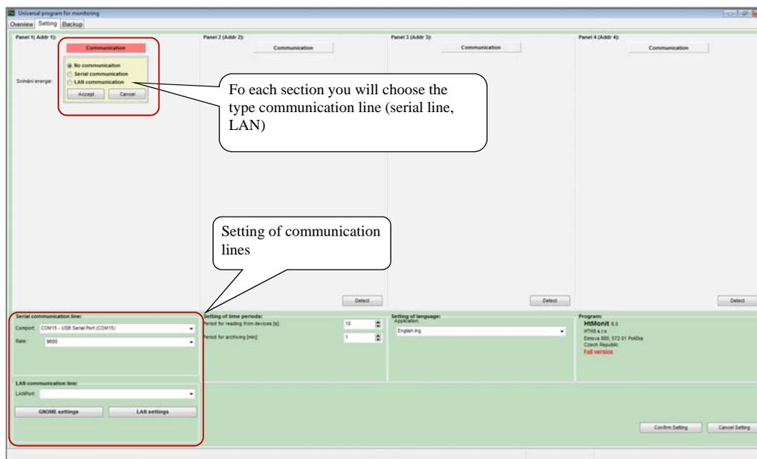
After setting of communication lines, you should carry out the detection of the linked devices.
