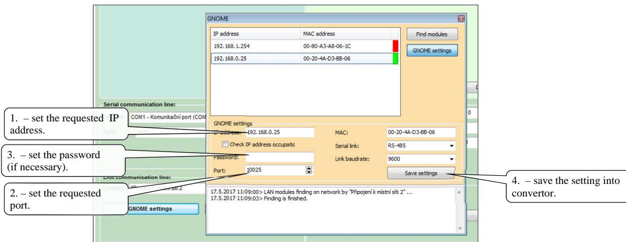
If the convertor GNOME is linked through sub-network and it is not displayed in the list (initial address of convertor is 192.168.1.254), you can proceed during its setting in the following way:
