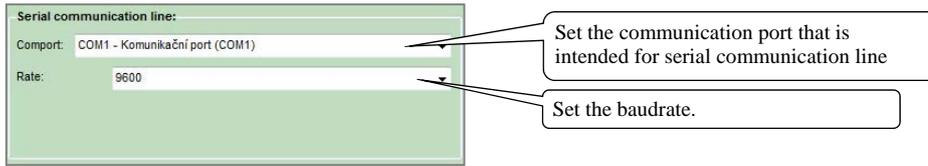
Setting of communication line must be confirmed by clicking the button „Confirm setting“.
