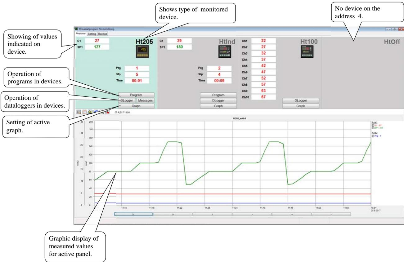
In the upper section of the window there are four separate sections displaying the indicated values for the connected devices.
