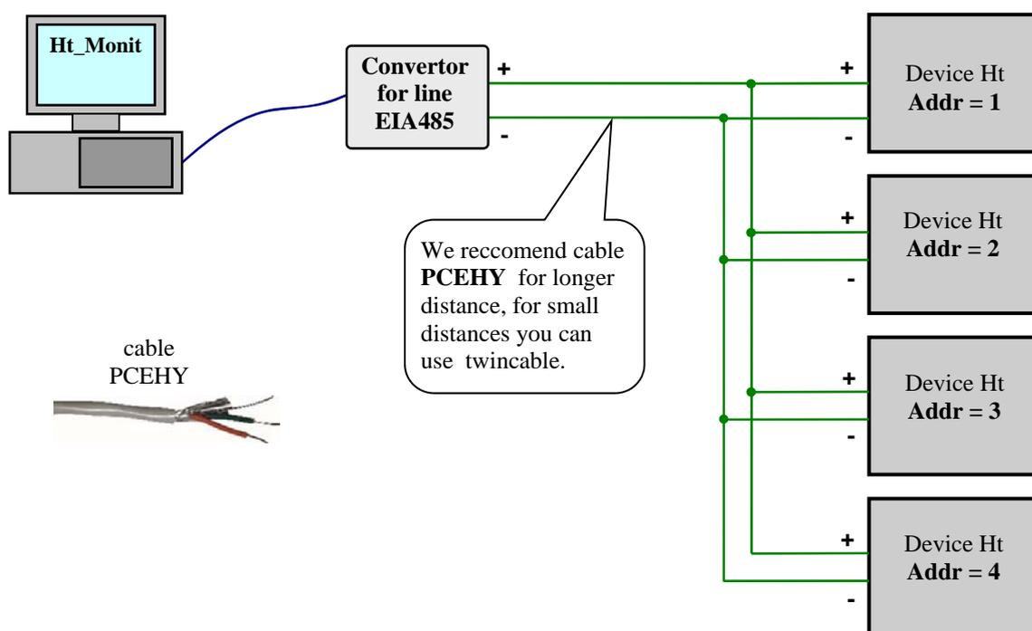
The devices listed in the following table can be linked on the communication line EIA485 via the description below:
