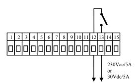
RELAY output is galvanicly isolated from the ground of the controller. For this output it is necessary to fix the wires in the way that in case of loosening the wire from the terminal the insulation would not be reduced between supply voltage and safety voltage.
