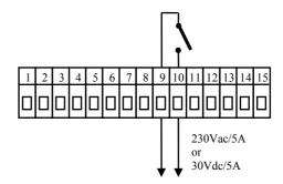
RELAY output is galvanicly isolated from the ground of the controller. For this output it is necessary to fix the wires in the way that in case of loosening the wire from the terminal the insulation would not be reduced between supply voltage and safety voltage.
