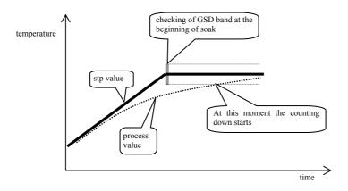
• GS typ = trak, GSD is active during the whole program. It means that the counting down is paused if the process value leaves the defined soak band GS dE.
