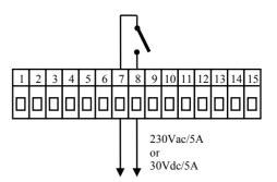
RELAY output is *galvanicly isolated* from the ground of the controller. For this output it is necessary to fix the wires in the way that in case of loosening the wire from the terminal the insulation would not be reduced between supply voltage and safety voltage.
