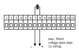
SSD is not isolated from controllers ground
