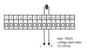
SSD is not isolated from controllers ground
