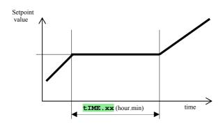
STP value of step SOAK is the same as the final STP of previous step. In case of starting a program the set point value is equal to the process value. Time duration of step is maximum 99 hours 59 minutes.
