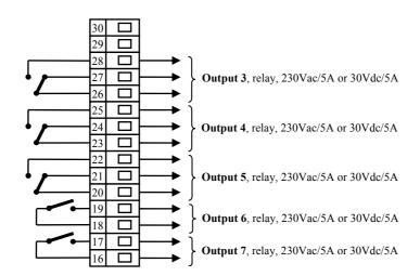
Relay outputs are galvanicly isolated from ground of controller
