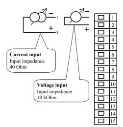
Measuring input is not isolated from ground of the controller
