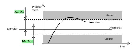
Parameters **AL Lo** and **AL hI** define low and high deviation from stp value at which alarm is active.
