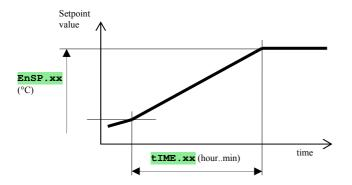
Initial set point value in step Stpt is the same as the final set point value of preceding (former) step. In case of starting a program the initial set point value is equal to the process value.
