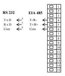
Communication is galvanicly isolated from the ground of controller
